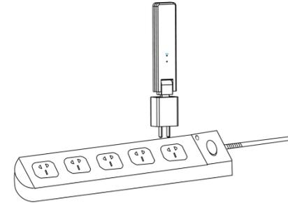
*Note: Please do not install the DTU directly above the metal or concrete to prevent the signal dilution.*
