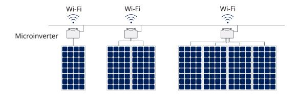
This manual is about Hoymiles 4-in-1 microinverter HMS-2000DW series. Its innovative 4-input design enables faster installation and lower cost, and makes the HMS-2000DW series a very cost-effective choice. Each microinverter connects to four PV modules at most with module-level monitoring, enabling greater energy harvest and easier maintenance.
