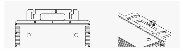
Route a continuous grounding cable through grounding brackets for each microinverter to the AC grounding electrode that conforms with local regulations.
