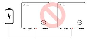
One battery cannot be connected to multiple inverters.
