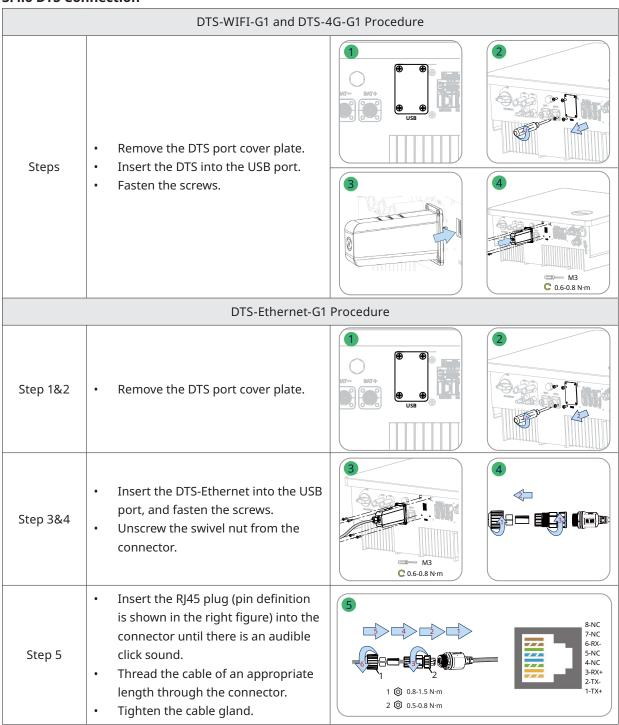
Note: The RJ45 plug with cable sheath cannot be inserted.
