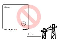
EPS port cannot be connected to grid directly.
