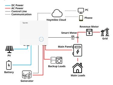
The HAS-LV series inverter can be connected to a battery and any grid-connected PV inverters to form a PV Energy Storage System (ESS). In the event of a grid outage, it can be used as an emergency power supply (EPS) through the self consumption of solar energy, as the grid-connected PV inverter can also work when it is connected to the GEN port even if there is a grid outage.
